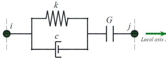
**Fig. 2 Viscoelastic impact model.**
