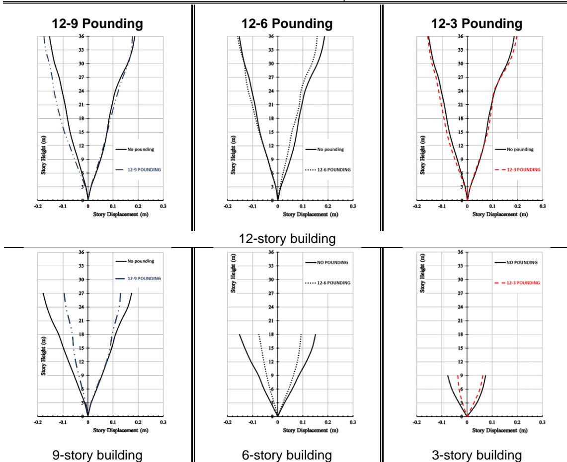
**Fig. 4 Displacement response envelopes for different Configurations.**
