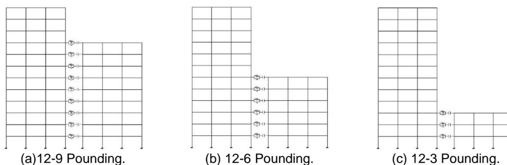
**Fig. 3 Different configurations of adjacent colliding buildings**
